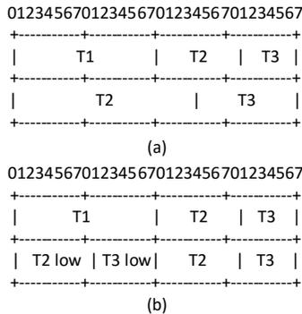
Fig. 3. The change of hash range after failure.
