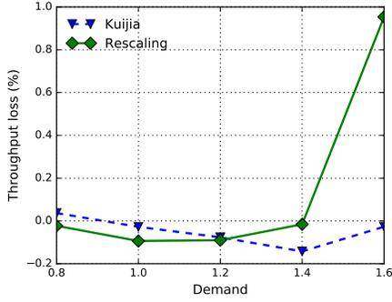
Fig. 7. Throughput loss of indirectly affected TCP flows.
