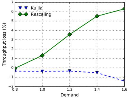
Fig. 6. Throughput loss of directly affected TCP flows.
